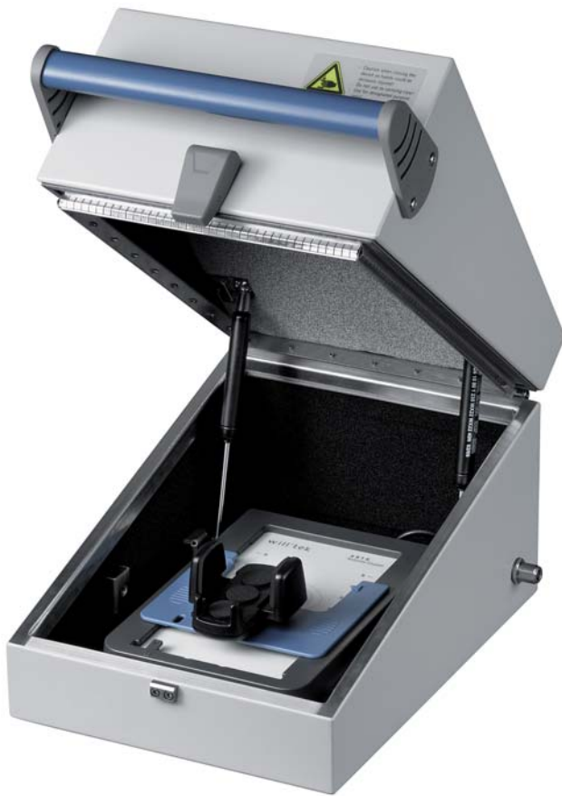
Figure 6: TETRA test chamber with aerial coupler
